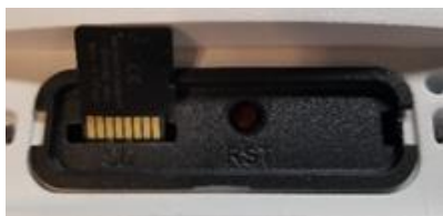
Insert SD card in Camera
