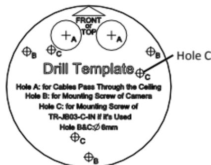
2. Drill holes with paster and use hole C.
