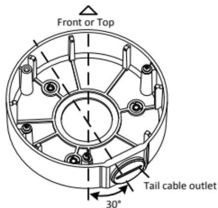
of the device is drawn from the outlet of the junction box.
