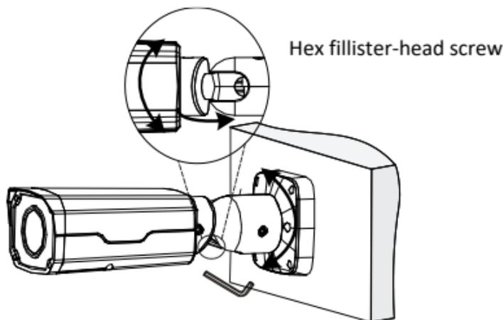
Loosen two hex fillister-head screws using a 4# hex L-key (that should be purchased separately) to avoid damaging the universal joint. Then adjust the camera to the desired monitoring direction. Fasten the screws to finish.
