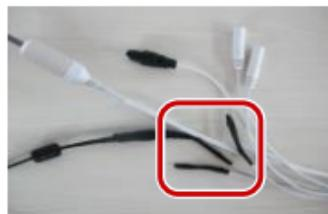
1. Connect the tail cables, and protect the cables and cable connections using insulating tapes. Then wrap all the tail cables together using insulating tapes.
