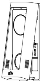
7. Tighten the anti-theft screws at the bottom of the device using the screwdriver.
