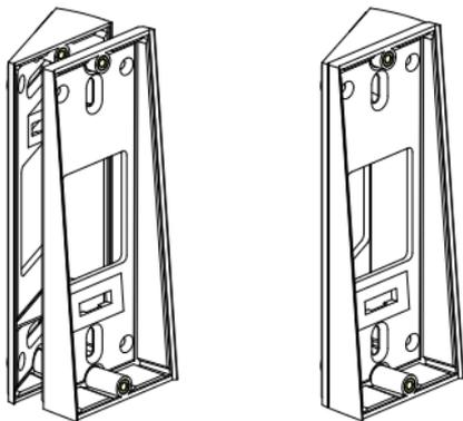
(2) Use the supplied 1.26" self-tapping screws when stacking brackets.
