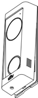
5. Secure the doorbell body to the bracket using the corresponding set screws.
