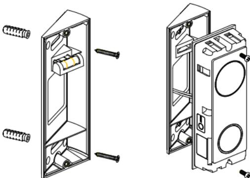
B. Install the angle adjustment bracket with 0.75" self-tapping screws.
