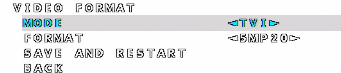
Figure 3-4 5MP Video Format Page (Default - Mode: TVI; Format: 5MP20)
